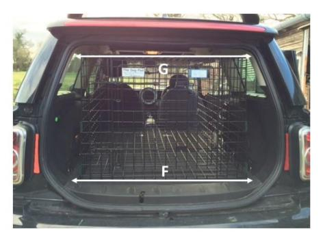
F – WIDTH OF THE CAGE FLOOR, THIS IS GOVERNED BY THE SPACE BETWEEN WHEEL ARCHES AND THE SIZE OF THE REAR DOOR, ACCOUNTING FOR ANY SHAPING AT THE CORNERS
